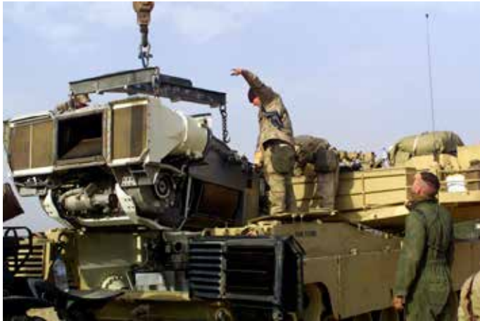
US Marines re-installing a gas turbine engine from an M1A1 Abrams tank-an example of western military gas guzzling.
